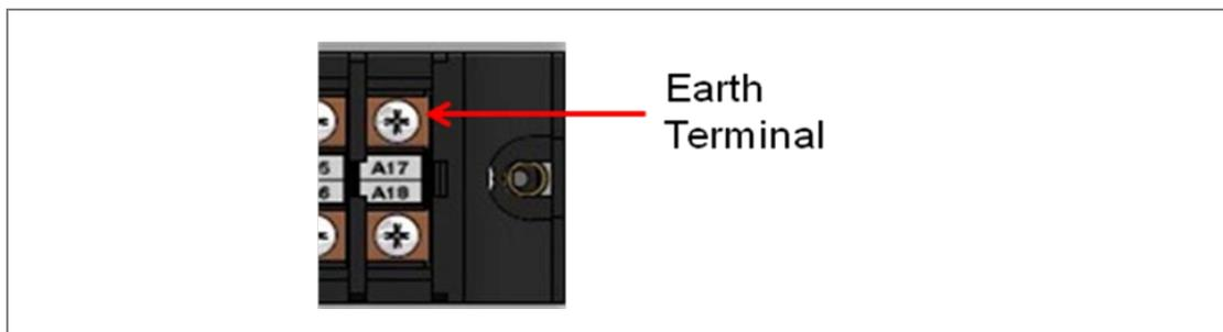
**Note:** To prevent any possibility of electrolytic action between brass or copper ground conductors and the rear panel of the product, precautions should be taken to isolate them from one another. This could be achieved in several ways, including placing a nickel-plated or insulating washer between the conductor and the product case, or using tinned ring terminals.
