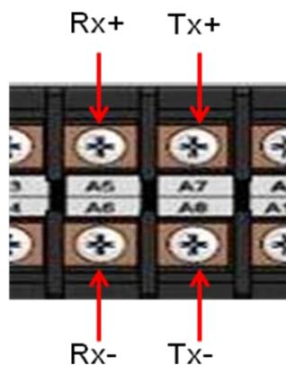
For connecting the RS422, use screened cable with a maximum total length of 1000 m or 200 nF total cable capacitance.
